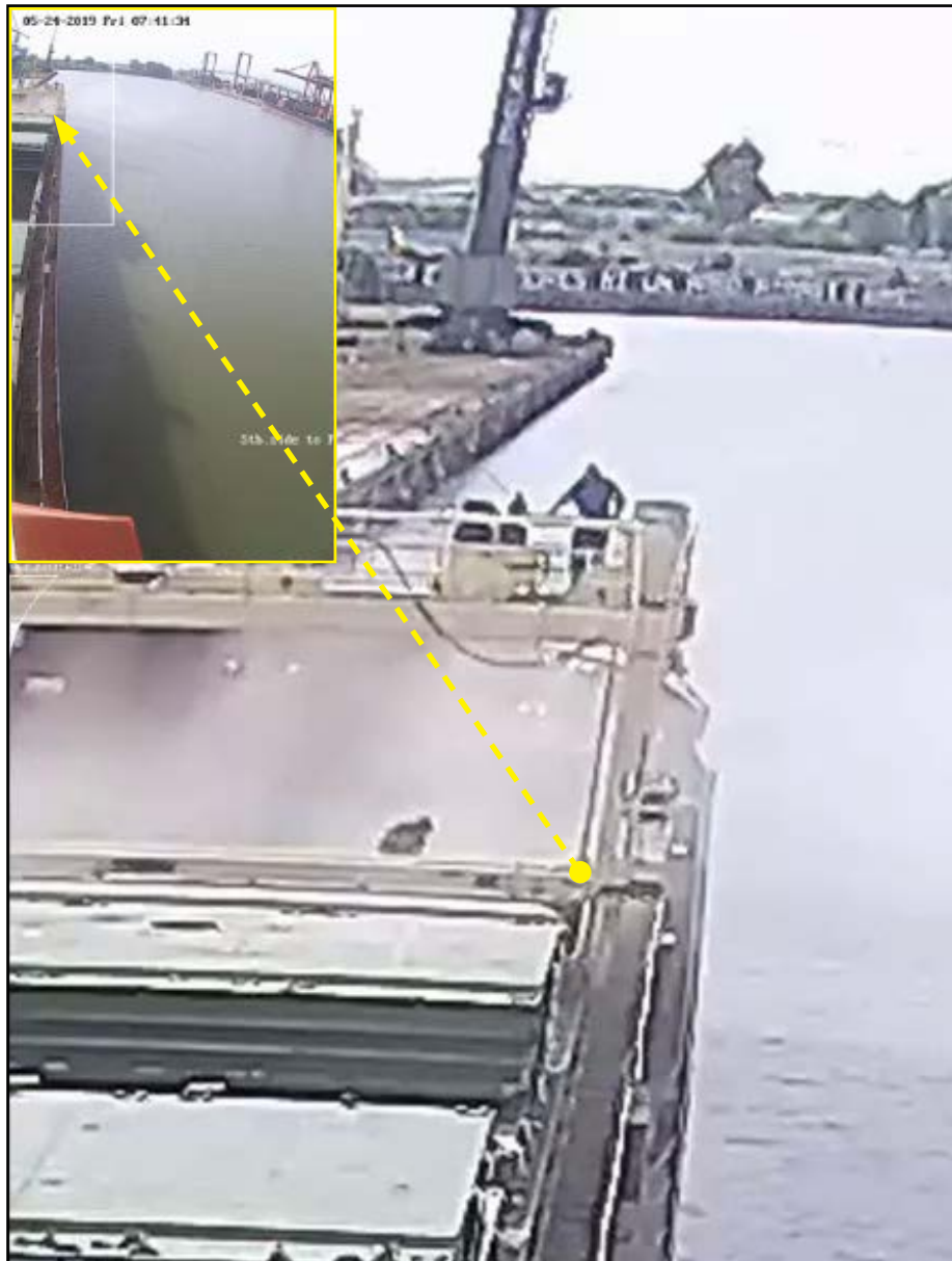
Figure 13: CCTV screenshot showing cement dust cloud
