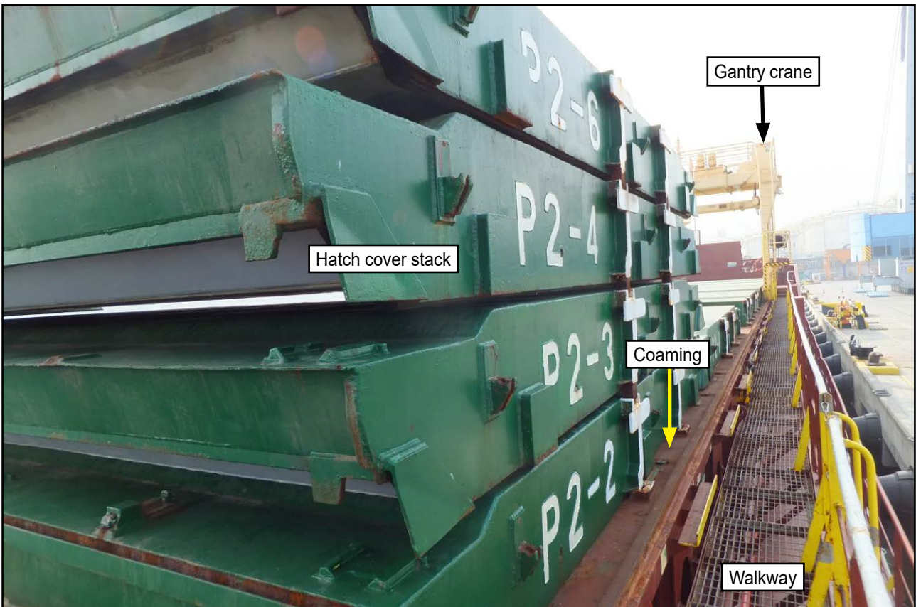
Figure 8: Starboard walkway showing stack of hatch covers and gantry crane
