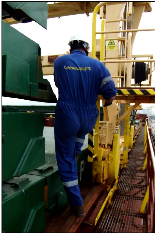
Figure 14: Climbing through the gap between the hatch covers and gantry crane (reconstruction)
