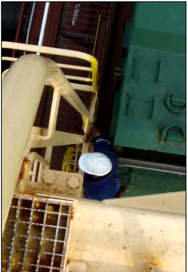
Figure 15: Reconstruction showing size of the gap between the ladder platform and the stacked hatch covers
