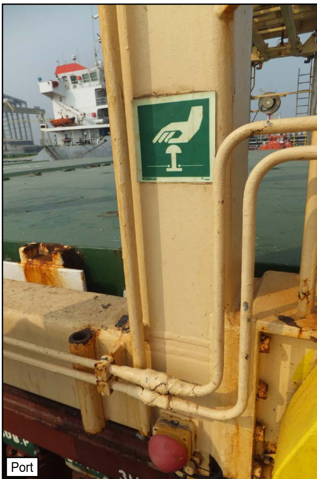
Figure 11: Gantry crane emergency stops
