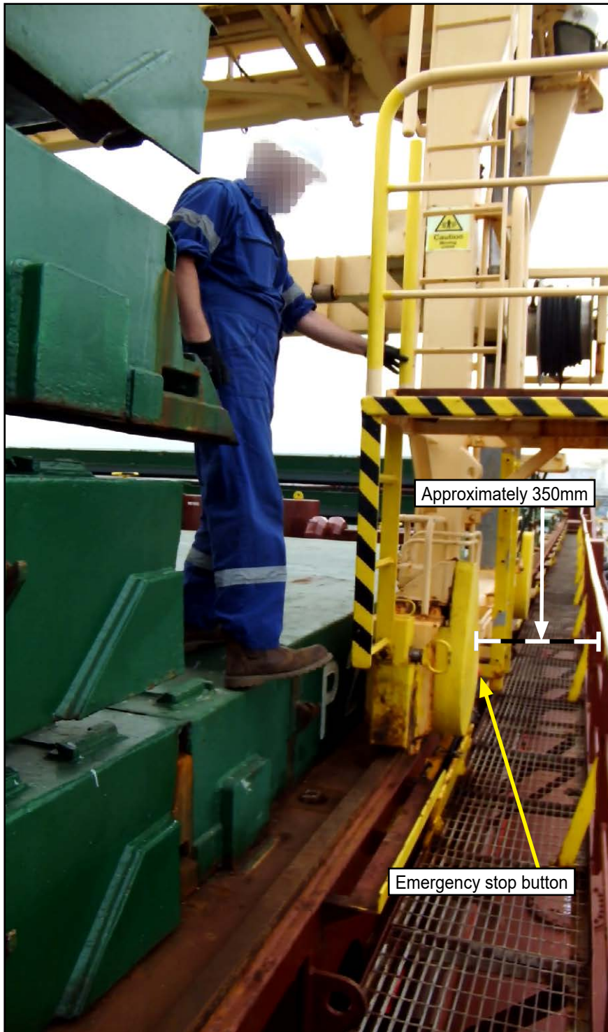
Figure 12: Access to starboard emergency stop
